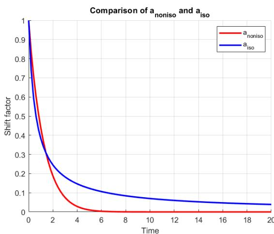
The relationship between **effective time and real time** was also explored to better understand the material's creep response under both isothermal and nonisothermal conditions.
