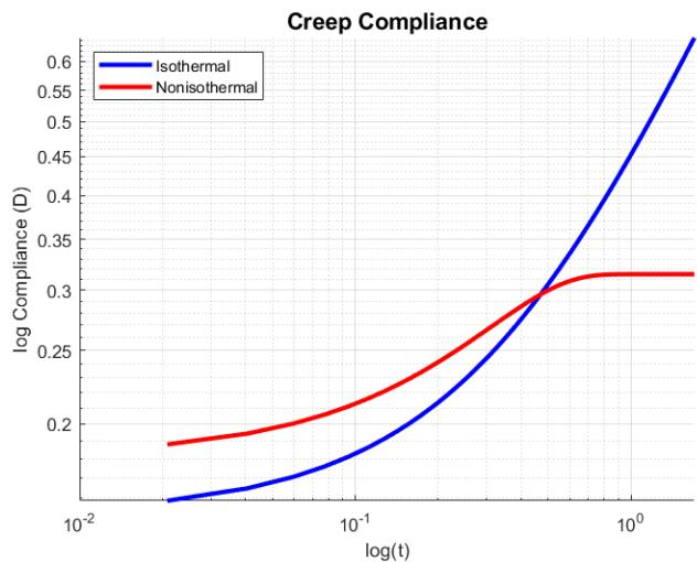
Finally, the comparison between effective time and real time for both isothermal and nonisothermal conditions highlights the influence of the aging process on the material's behavior with respect to the time scale under varying thermal conditions.
