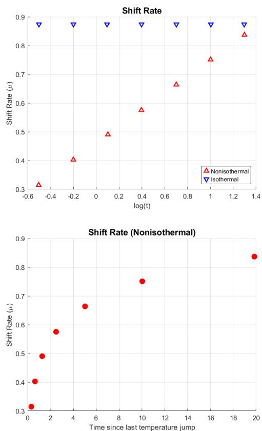
The fitted shift factors for isothermal and nonisothermal aging are also provided, highlighting the distinct behaviors of the material over time.
