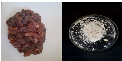
Figure 3: Representative visual aspect of cashew gum before (left) and after (right) purification by dissolution in water followed by precipitation with ethanol, centrifugation, filtration, and milling. [15]
